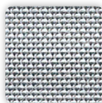
Uginox Linen (2J) Etched linen finish obtained by cold rolling with special rolls, followed by a final anneal. For internal use.
